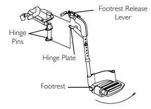
FIGURE 6.1 Installing/Removing Footrests - Phal4A, 70° and pw93
